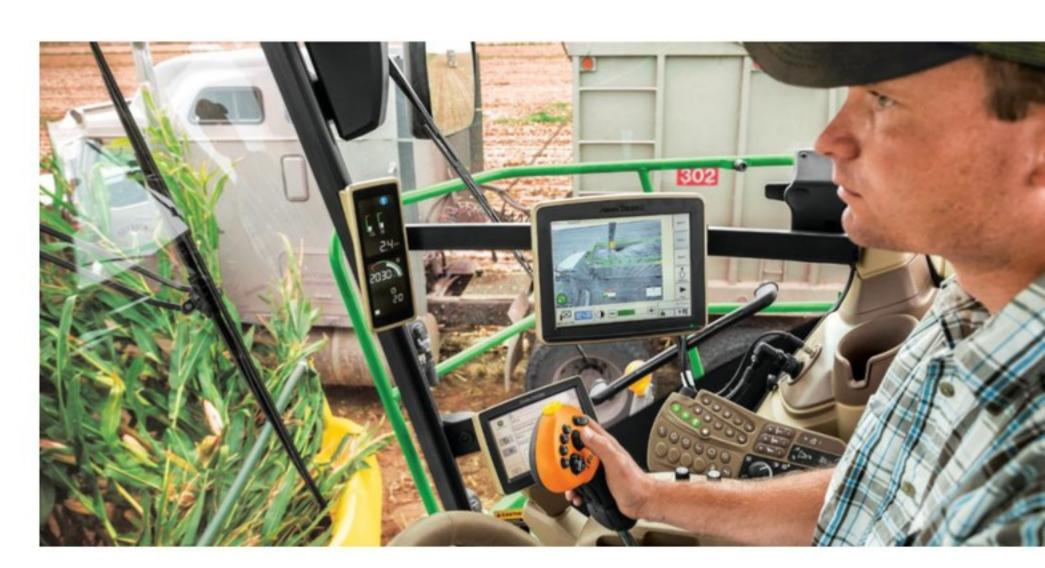
Ensure your crop doesn't end up on the ground. The optional Active Fill Control uses cameras with 3D capability to automatically detect the crop transport truck or trailer, and fill it evenly and without spillage. As the camera detects a truck, it automatically begins tracking with the spout. Then it controls the rotation and cap position of the spout until the truck is filled.
