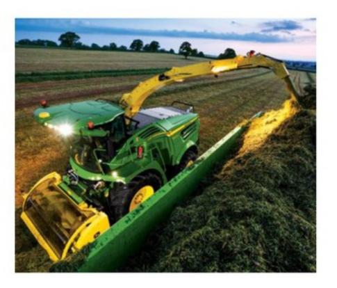
The available Automatic Spout Positioning allows you to store up to three spout positions. The spout height, rotation, and cap position can all be preset and stored. With a spout reach between 15 (standard), 19.2 and 22 (optional) feet, 210 degrees of rotation and standard hydraulic raise and lower, you'll find maneuvering the spout just where you need it to be simple.
