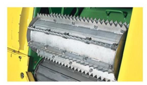
Save money with an upper front feedroll that features **bolt-on serrated or straight replaceable teeth bars** specifically designed for high wear conditions, sandy soil, and high-yield corn.
